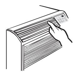
Remove the front grille to adjust the vertical louvers side-to-side to direct the air left or right.
