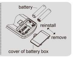
3. Reinstall the cover of battery box.
