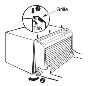
Hook the tabs on the front grille even with the tabs on the case and snap into place. Replace the screws and filter. Refer to Page 2, Figure A.
