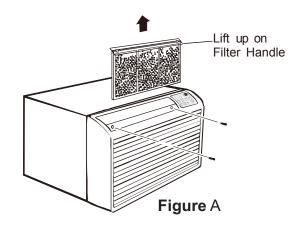
The front grille can be removed for more thorough cleaning or to make the model and serial numbers accessible. To remove, pull the filter out and remove the two grille screws.
