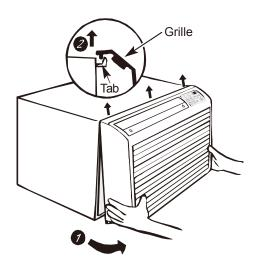
Pull the grille out from the bottom and lift up from the tabs on the top of the case.
